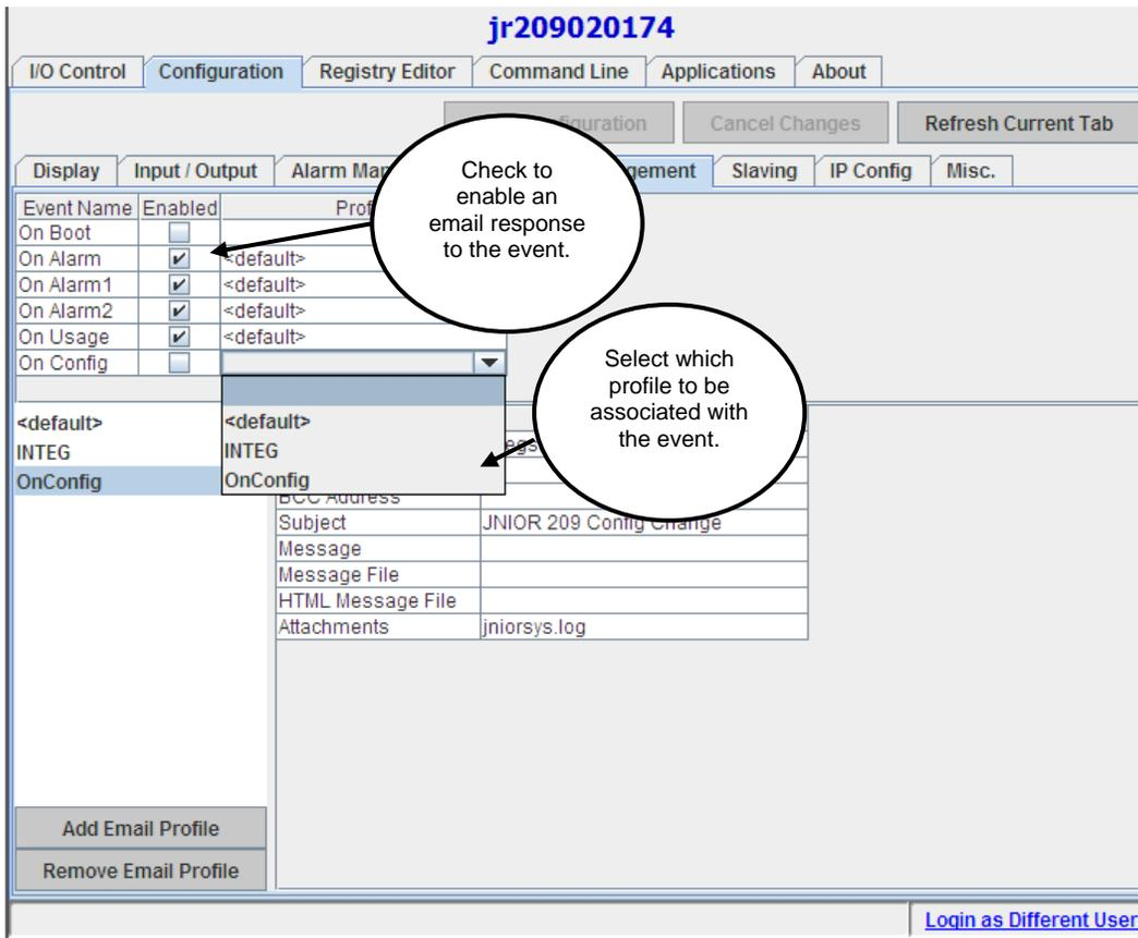
**On Boot** – When “Enabled”, JNIOR will send a notification to the specified Profile upon complete of the JNIOR boot sequence. The jniorboot.log file can be an attachment in the e-mail profile.
