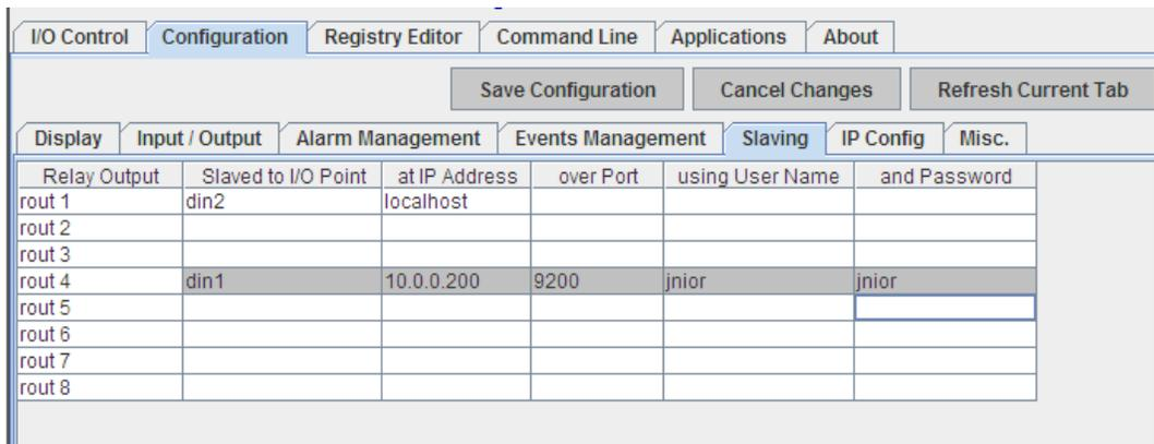
After your reboot, the slaved output will be indicated on the JNIOR Web page. The master I/O point will be indicated and the IP address of the remote JNIOR. The Toggle button for this output will be disabled.
