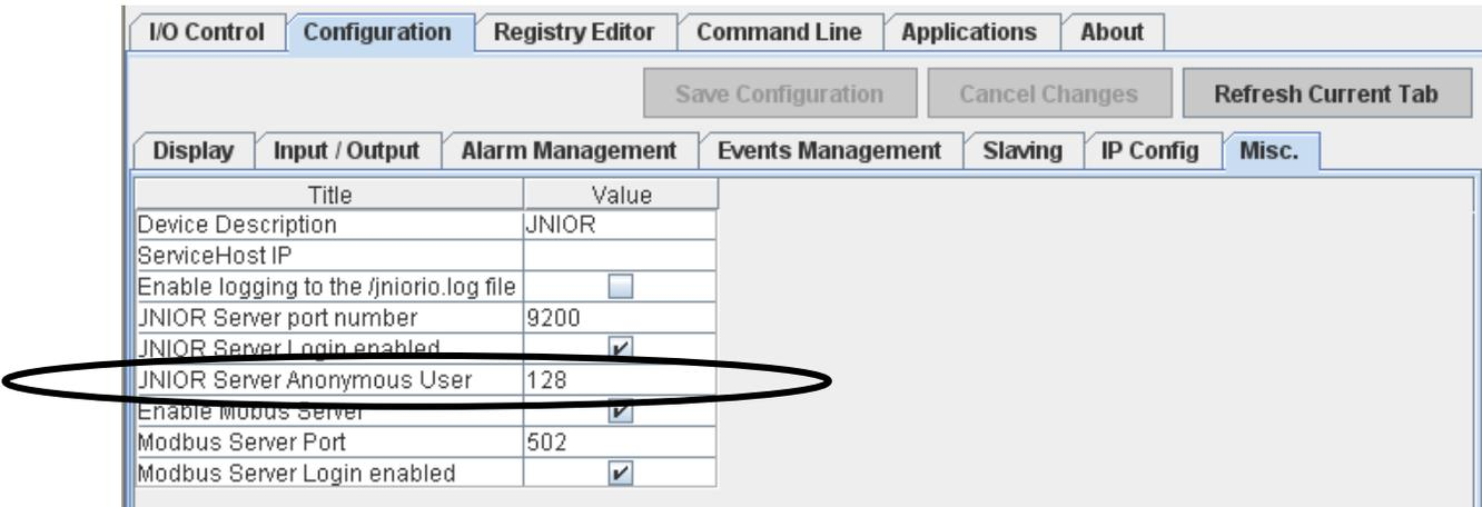
Even though the web page automatically logs in at the defined rights level, you can click on the “Login as Different User” text in the lower right hand corner of the web page to get the login and password prompt. You can then enter any valid username and password and the web page will give you the appropriate rights and capabilities. You can disable automatic login by going to the Configuration/Misc Tab and deleting the value saved in the JNIOR Server Anonymous User field.
