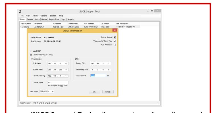
JNIOR Support Tool—allows you to easily configure and manage your JNIORs via the Ethernet network
