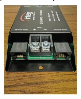
Once the dimmer is connected on the sensor port, a green LED next to it will light up. Next, the dimmer will need external power to light the LEDs. A 5-24 volt DC power supply must be connected to the dimmer module on the + - INPUT terminals to power the LED strip lights, which are located between the sensor ports. The voltage you apply should match the voltage required by your LED strip lights.
