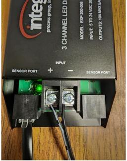
You can control up to 3 different white LED strip lights or 1 set of color (RGB) LED strip lights per LED Dimmer module. Each channel can handle up to 10 amps, handling up to 30 amps total. Each channel uses Pulse Width Modulated (PWM) control to vary the LED strip lighting intensity between 0 and 100%. The voltage is controlled on the **negative side** to conform with most standard LED strip lights.
