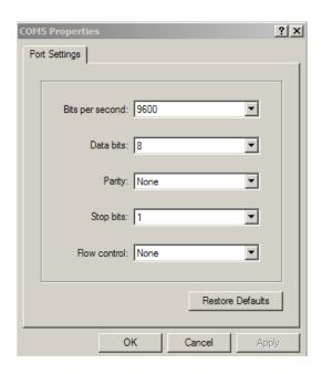
After connecting a cable from your COM port to the JNIOR Auxiliary Serial Port and opening HyperTerminal, you can issue control commands and also receive status messages. An example is as follows:
