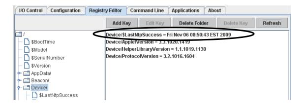
You can also force the JNIOR to sync its time with the currently entered NTP server or a temporary one by using the date command from the Command Line tab (or a Telnet session or HyperTerminal session) as follows:
