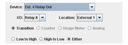
When using an external relay output in an 'event', the user must select whether the expansion module to be used is External 1 or External 2. Each output is lettered A, B, C or D on the expansion module label and the user must select one of these as the trigger. However, when using the 4 Relay Output Expansion Module outputs as part of an 'action', they are numbered 9 through 16.
