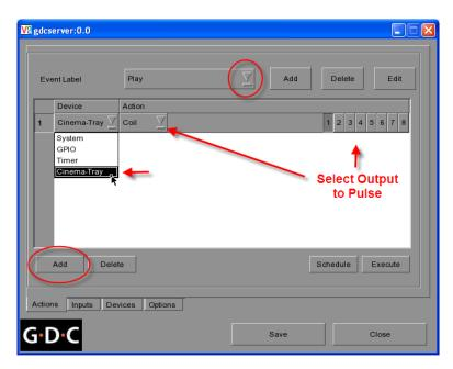
If you select the LEVEL action, the GDC will either 'close' (turn on) the relay output or 'open' (turn off) the JNIOR relay output.
