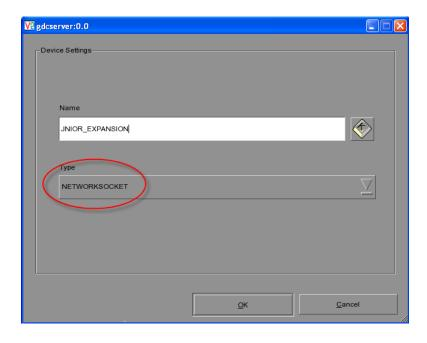
You will have to configure the Network Socket Connection to match the Serial Control PLUS settings.
